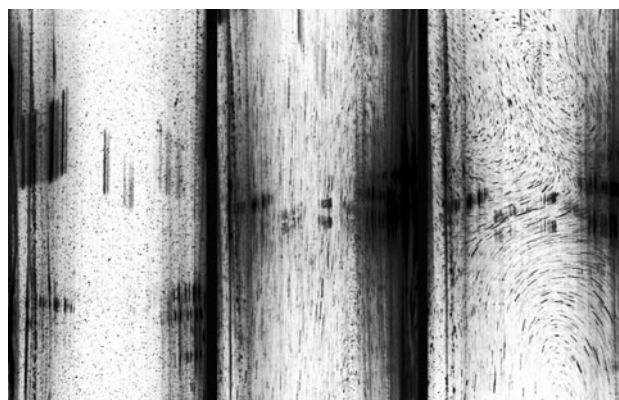
Fig. 5 Long-time exposure of tracer particles in a 5 cm \times 10 cm section of the water column; left , without temperature gradient; center , convection at a temperature gradient of 0.4 K/m; and right , at a temperature gradient of 2 K/m
